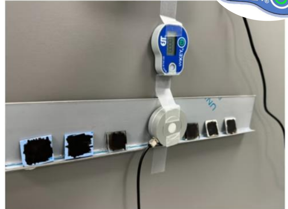
Figure 4. Coupons of vinyl, glass and steel with Aspergillus brasiliensis spores inoculated. The UVKEY and ILT2400 dose meter are in place and set to zero prior to start.
