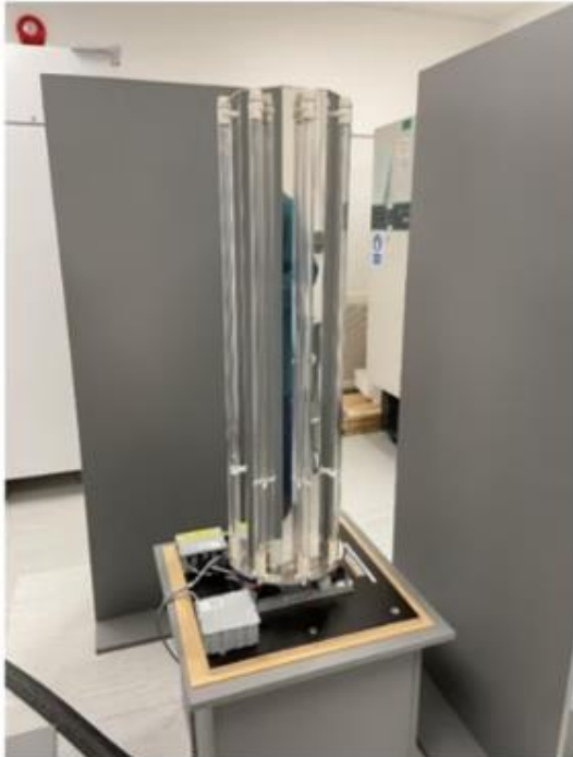
Figure 1a. UVC Tower set up in the laboratory. The boards in the room were to attach the coupons two metres distance from the light Figure 1b. The black cloth was used to protect the control coupons from the light.
